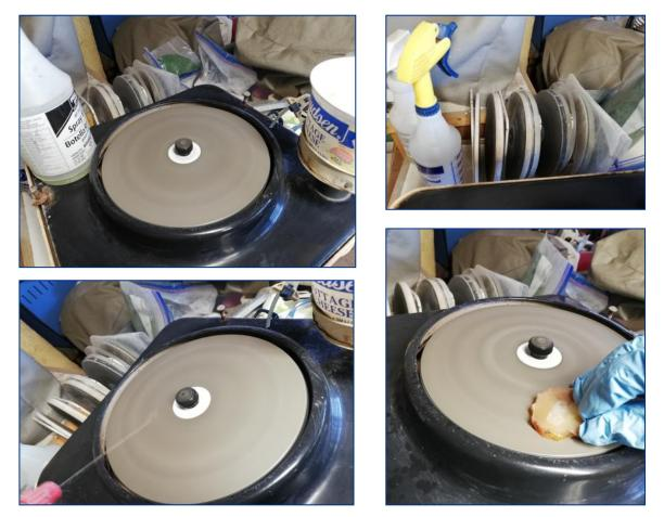
The club have a flat lap grinder polisher at the workshop for members to use. This lapidary machine comes with several diamond lapping discs. There is a small drip tank to hold water. We can also spray water directly on the disc when using the machine. This flat lap can grind and polish a flat surface on your gemstone; it can also be used for simple faceting.
