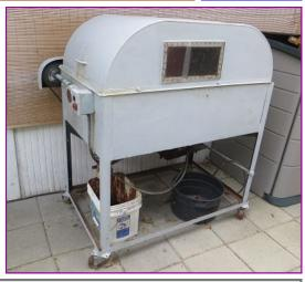
Sometimes it's just fun to cut open a rock you pick up in the field and see what is inside of it. A lot of rockhounds do that. A small rock saw or tile saw can be used to cut smaller rocks. A larger slab saw is required to cut larger pieces of rock. For most lapidary work, a 16 inch slab saw can do most of the tasks, and to cut open a good size of geodes or nodules.
